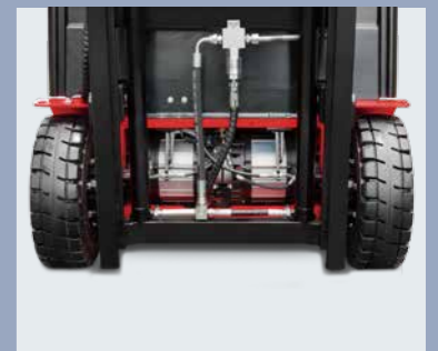
Front dual separated motors
