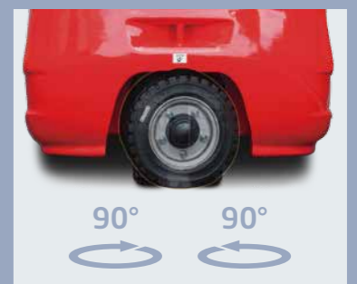
The small turning radius is suitable for narrow aisle
